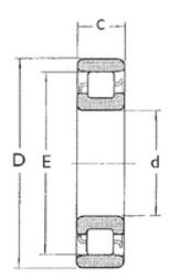
N308 Bearing 2D drawings and 3D CAD models
