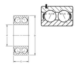
Timken 5306WG angular contact ball bearings
